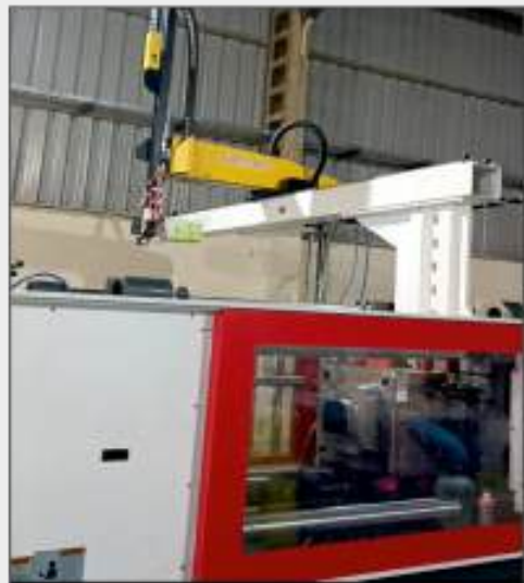
In Mould Labeling (IML) of Plastic Jars for Packaging Industries Using Robotics
