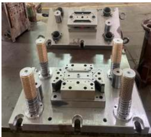
Press Tool for Ammunition box H60 for Ordnance Factory Bhusawal.
