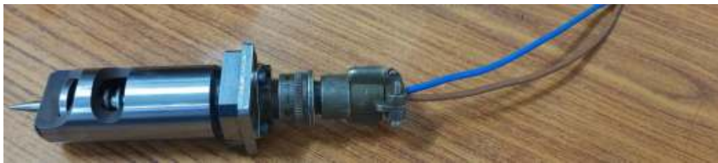
Manufacturing of Firing Pins for AK 360 Gun for Naval Armament Inspectorate, Khamaria Previously it was imported from Russia.
