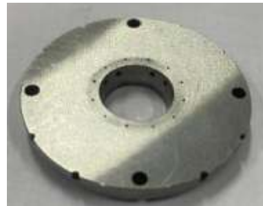
Manufacturing of Face Plates for Balancing Machine of Turbo Chargers for Cummins Technologies India Pvt. Ltd., Pithampur, Previously it was imported from USA.
